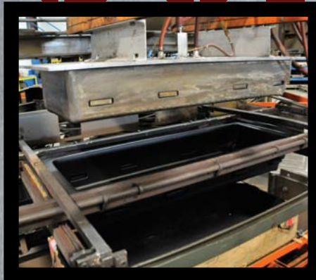
Pictured: Vacuum mold for keyboard case.
